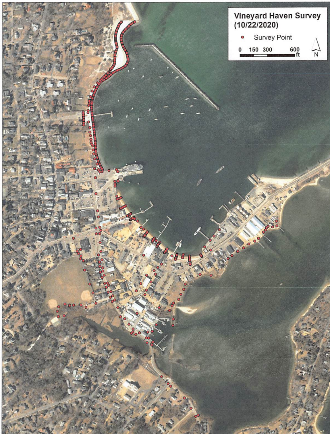
Figure 1 Map of downtown Tisbury with surveyed points from the 10/22/2020 survey marked with a red dot. The survey will help identify storm tide pathways that can be mitigated for with the site specific conceptual designs.
