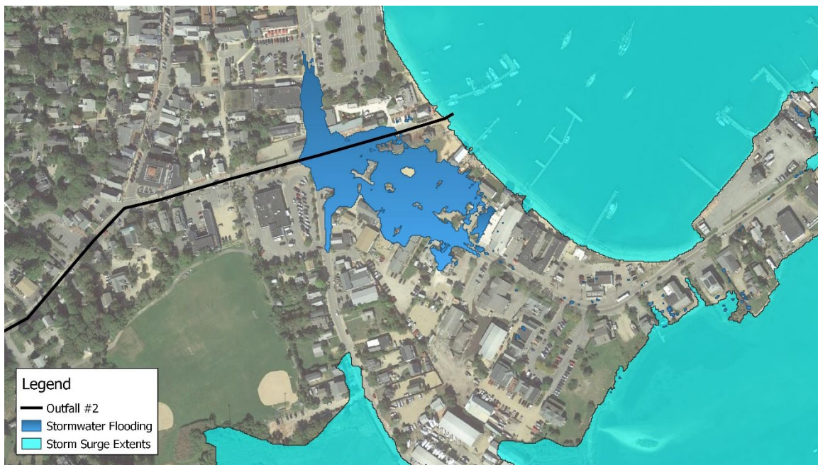
Figure I.18 Location of coastal storm surge and stormwater flooding during a 3.5-foot NAVD flood elevation. Stormwater primarily will flood around the five corners intersection of downtown.
