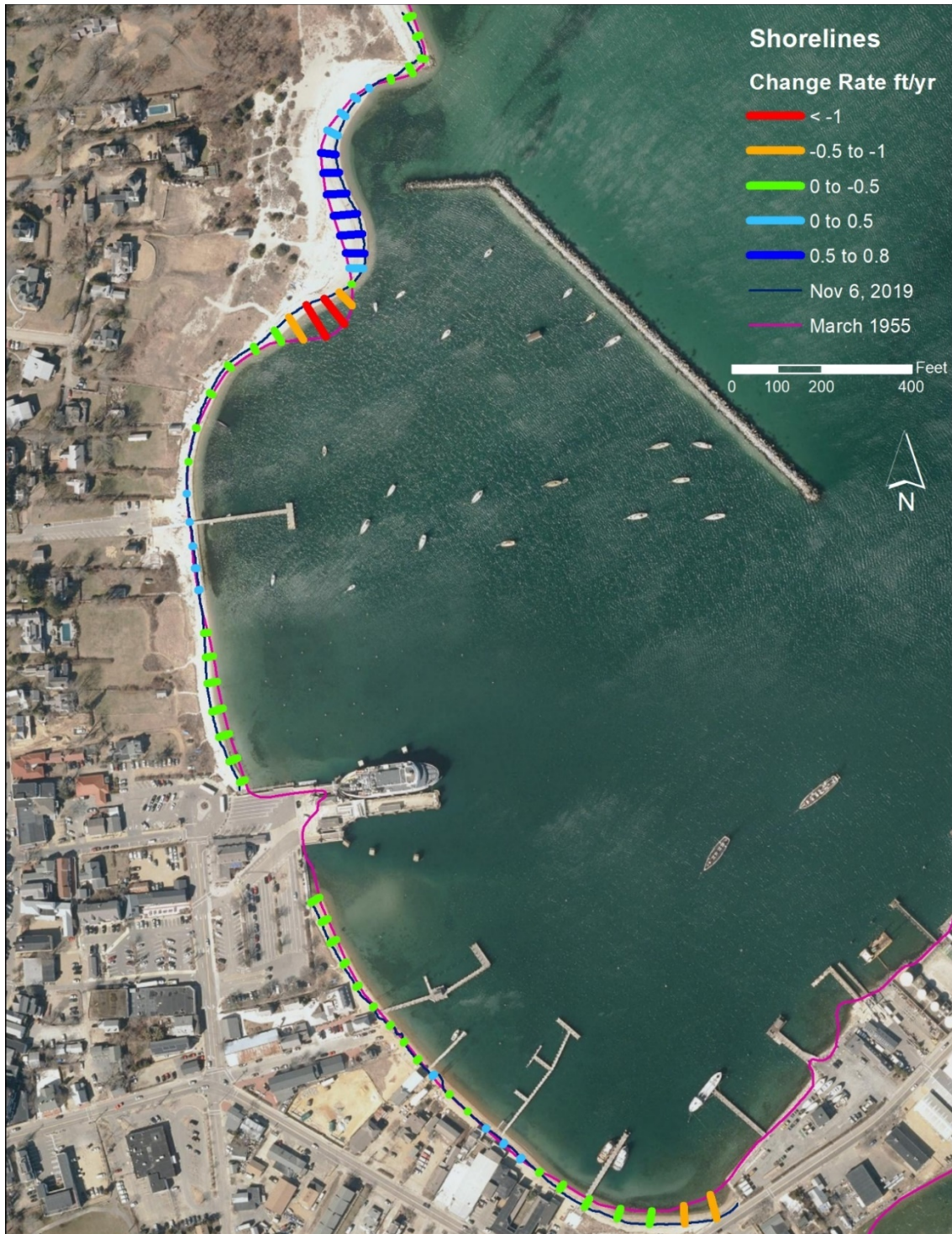
Figure A.5 Results of shoreline change analysis using the March 1955 and November 2019 RTK-GPS shorelines. Color bars indicate a range of shoreline change computed along Vineyard Haven shoreline. Negative rates indicate erosion, and are represented by the colors yellow, orange, and red. Areas of accreting shoreline are indicated by green and light and dark blue.
