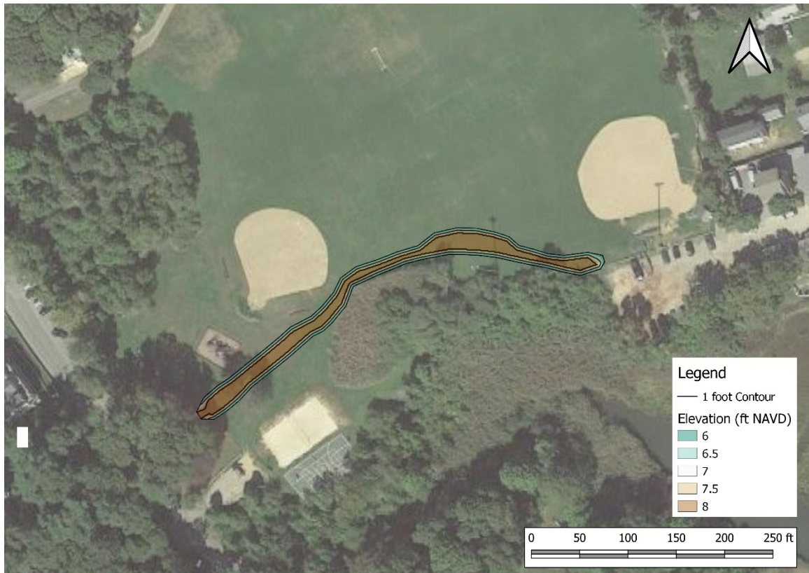
Figure C.7 Color contour elevations of the berm design for Veterans Memorial Park.
