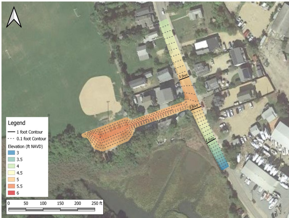
Figure C.6 Color contour elevations of the Lagoon Pond Road design.
