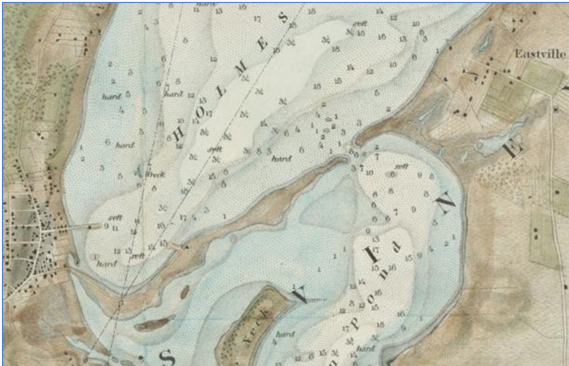
Figure I.19 Section of the 1847 U.S. Coast Survey navigation chart for Holmes Hole (Vineyard Haven Harbor) illustrating the natural deep channel along the length of the Harbor, as well as early pier development in the vicinity of the Packer Facility.
