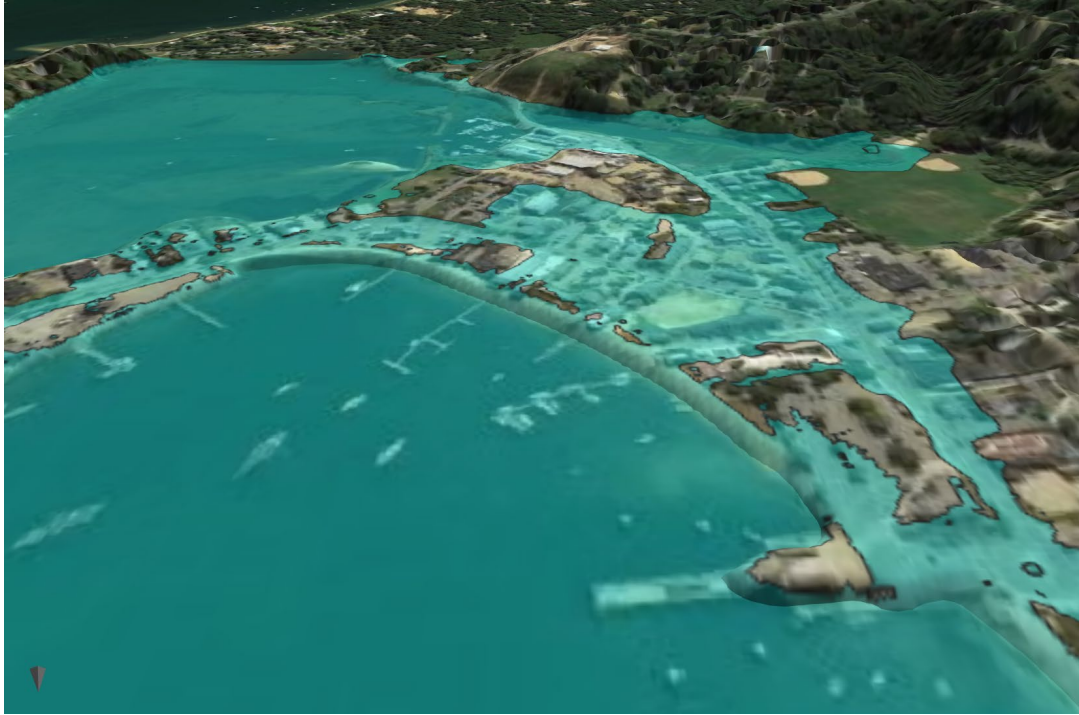
Figure 3 Flooding extents downtown during a 4.5-foot NAVD storm water level if no resiliency measures are incorporated in to Vineyard Haven.
