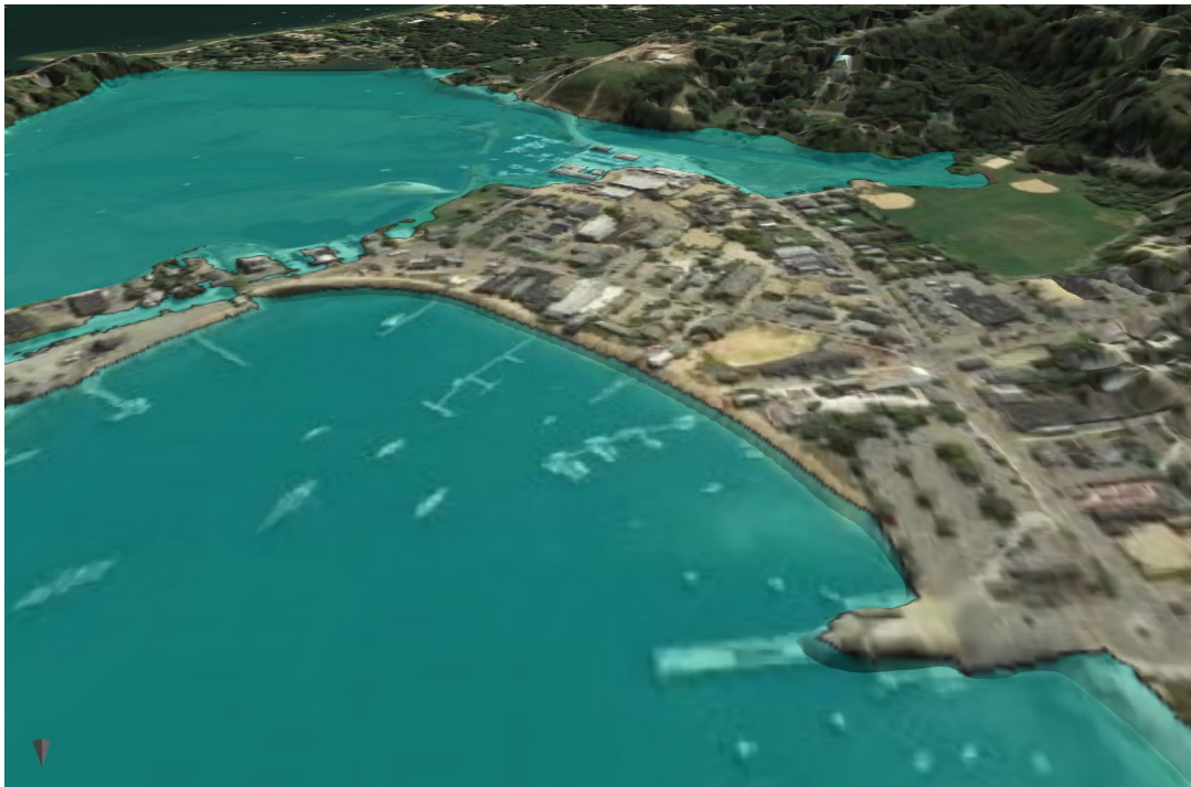
Figure 4 Flooding extents downtown during a 4.5 foot NAVD storm water level if all resiliency designs are accounted for.
