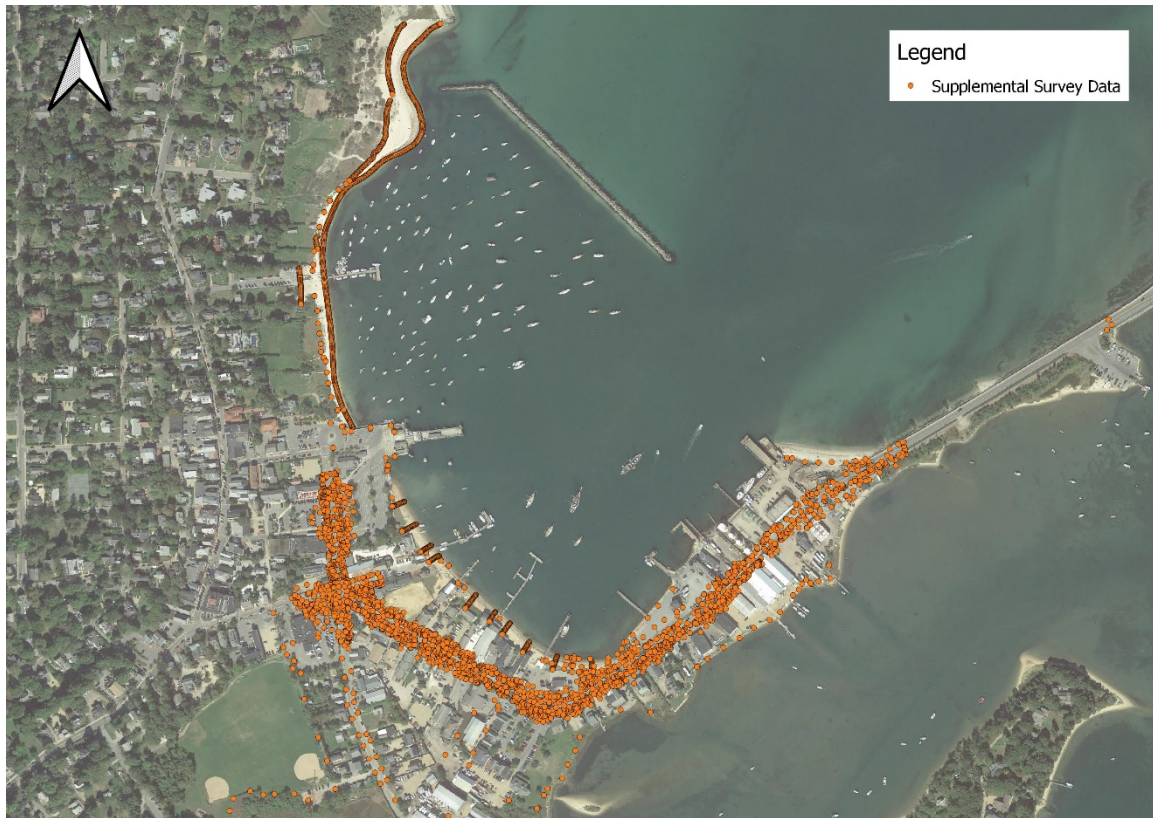
Figure I.5 Location of all additional survey points collected to compliment the 2018 LiDAR dataset.
